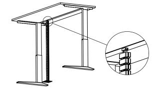
Locate a horizontal metal section of the desk frame where the magnet can be attached. To test the strength of the attachment, pull the assembly straight down. If the attachment of the magnet is not secure, test another location along the metal frame and repeat the test.
