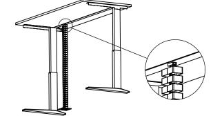
Assemble the E-Mag-2B onto the 2 x Pins of the Cable Snake Chain Link.
