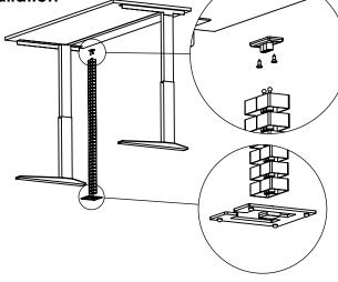
Fix the Easy-Desk-2B with the 2 x screws provided. Once secure, insert the Pins of the Cable Snake Chain Link into the Easy-Desk-2B. Force may be required to engage the Pins into the bracket. Apply the same technique to assemble the Easy-Floor.
