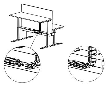
Position chain Link into desk channel. Use E-Mag to secure Chain Link into the channel. (Desk Channel cut away for clarity)
