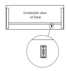
Choose the location of the Easy-Desk-2B on the underside of the Desk. Ensure the Chain Links are straight and locate over an opening in the channel cover plate (if present).
