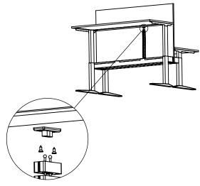
Fix the Easy-Desk-2B with the 2 x screws provided. Once secure, insert the Pins of the Cable Snake Chain Link into the Easy-Desk-2B. Force may be required to engage the Pins into the bracket.
