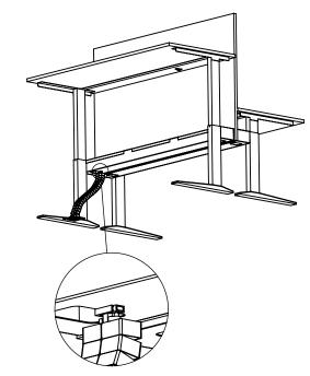
Locate the magnet to the underside of the channel near the opening where the cables enter / exit the channel
