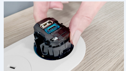
Unwrap and insert the new TUF cartridge, paying close attention to the orientation of the cartridge to the blue housing.
