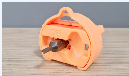
Insert the 'snake eye' bit into the tool as shown.
