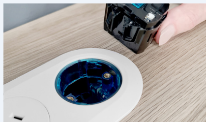
Unwrap and insert the new TUF cartridge, paying close attention to the orientation of the cartridge to the blue housing.
