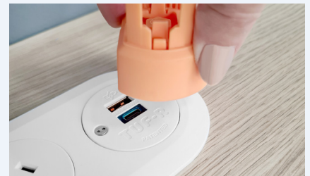
Use the tool to unscrew the 'snake eye' screws.
